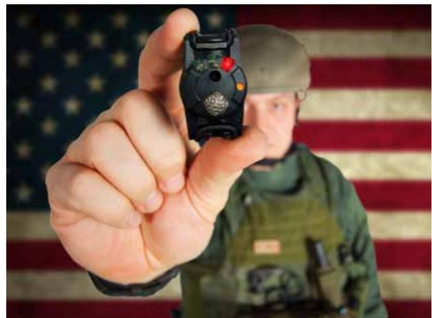
Image 3: Blackbox Biometrics B3 Blast Gauge showing activation of Red Indicator Light. (Photograph courtesy of BlackBox Biometrics Inc.)
